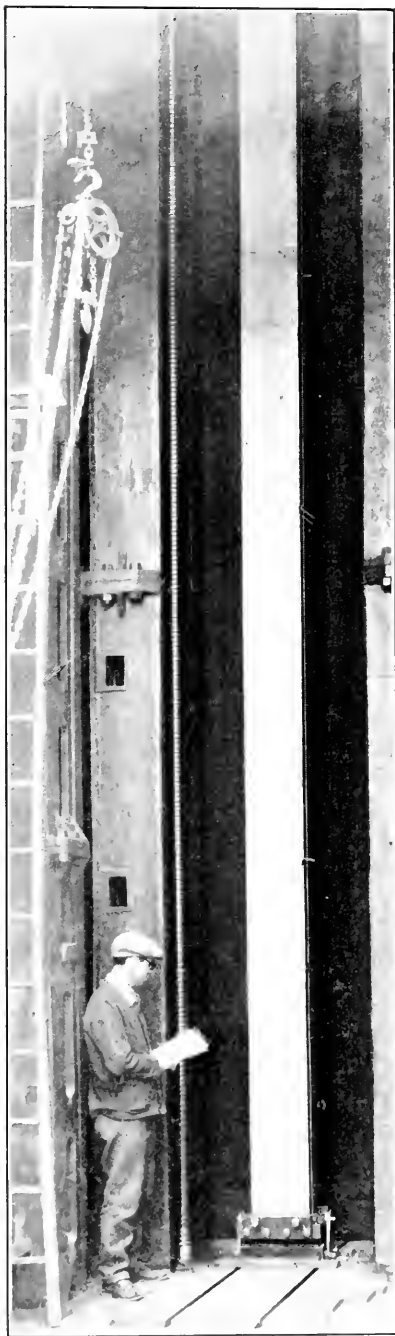
A long column mounted upon the special roller bearings preparatory to test in the Forest Products Laboratory 1,000,000-pound timber-testing machine
